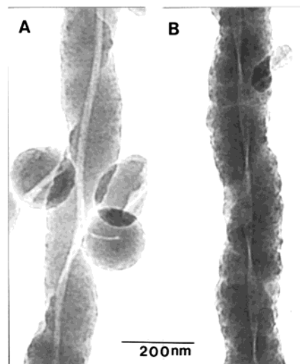
Figure 3. TEM pictures of the silica obtained by sol-gel transcription in (A) left-handed 1+2 (1:1 wt %), and (B) right-handed 3+4 (1:1 wt %) organogels.
